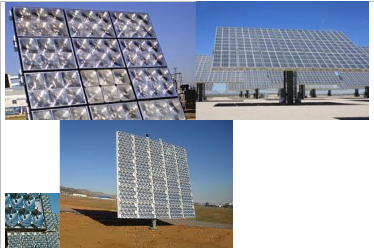
Figure 4-1: Example of Concentrated Photo-voltaic technologies (Bullis, 2011).
